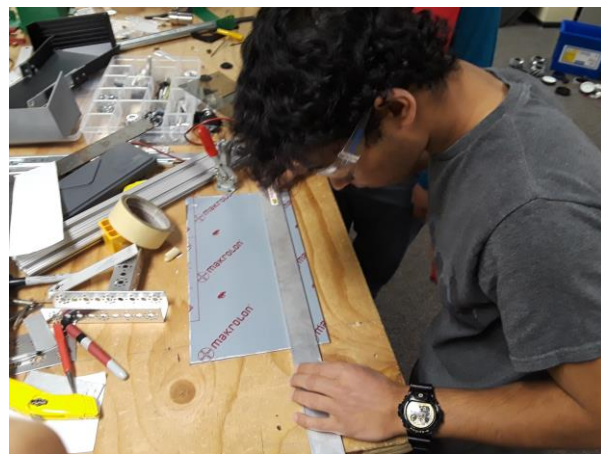
Ronin marking lexan for the robot number plates
