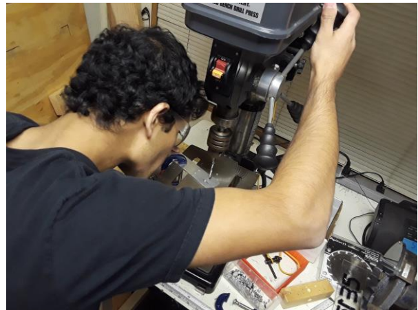
Ronin drilling holes for the lift mechanism
