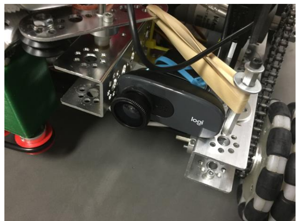
Webcam with wide angle lens for mineral detection
