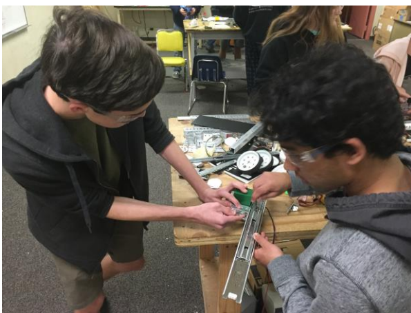
Alex and Ronin measuring holes for the linear slide
