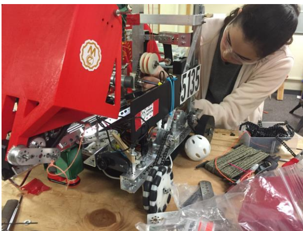
Sam installing the chain for the revised lifter gear ratio
