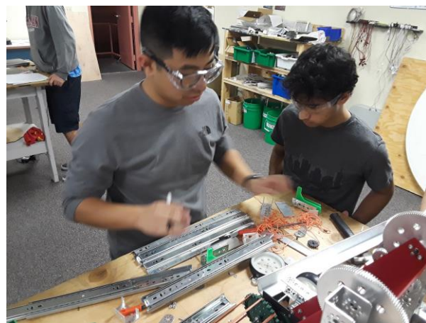
Noah and Ronin marking holes for linear slides
